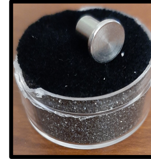
Stainless steel coupon (surface for biofilm)
